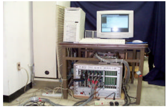
Fig. 9. VME-bus based robot hand control system.
