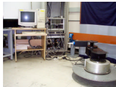
Fig. 4. Two link direct drive robot and its control system.
