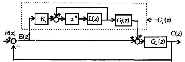
Fig. 1. Block diagram representing two conventional repetitive control systems: (a) a prototype single repetitive control system  $[L(z)=1]$ ; (b) a modified single repetitive control system  $[L(z)=q(z)]$ .
