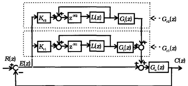
Fig. 2. Block diagram representing two proposed dual-repetitive control systems: (a) a prototype dual-repetitive control system  $[L(z)=1]$ ; (b) a modified dual-repetitive control system  $[L(z)=q(z)]$ .
