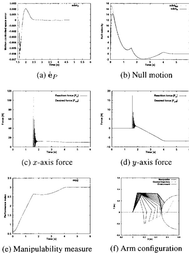
Fig. 4: Contact transition control performance
