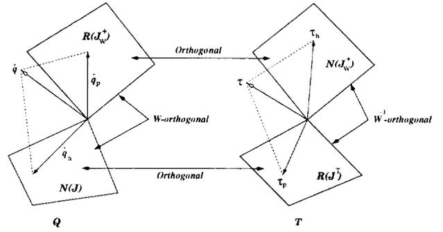
Fig. 1: Weighted joint space decomposition
