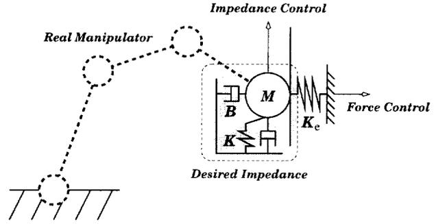
Fig. 2: Fundamental idea of hybrid impedance control
