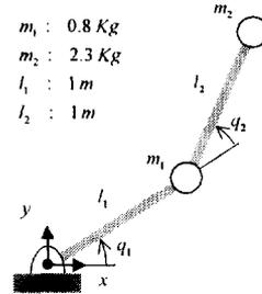
Fig. 6 A two DOF planar type robot manipulator
