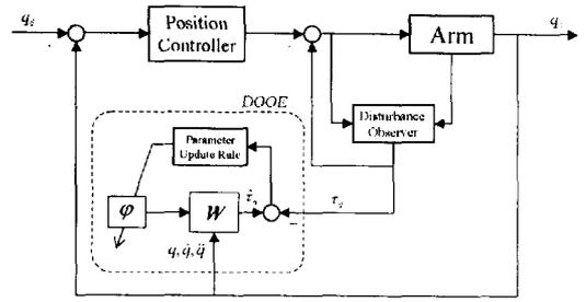
Fig.3 The block diagram of DOOE
