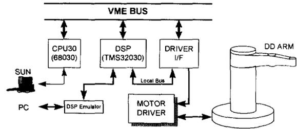
Fig.10. Experimental Setup
