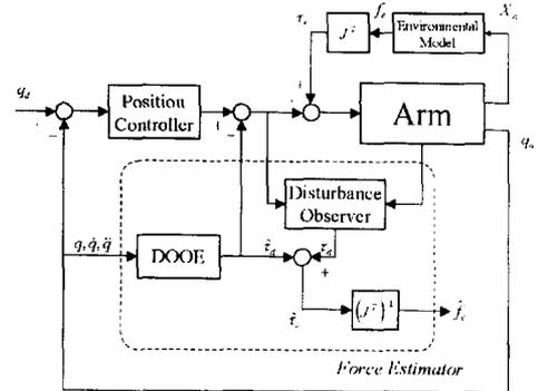
Fig.4 The block diagram of force estimator
