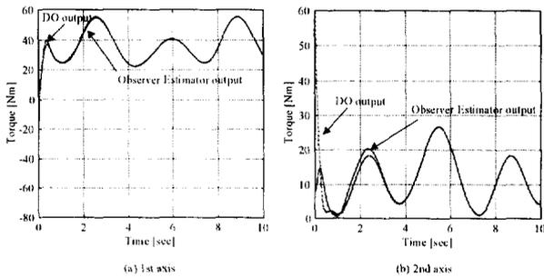
Fig. 8 The output of DOOE and the output of disturbance observer
