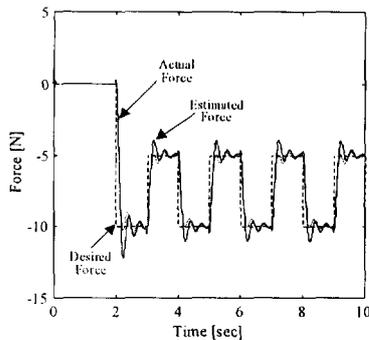
Fig. 9 The force response using the proposed force estimator
