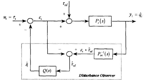
Fig.2. A structure of disturbance observer.
