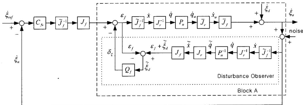
Fig. 4. The block diagram of proposed visual servoing method using disturbance observer
