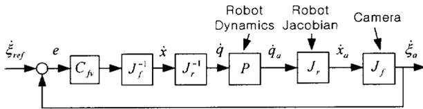
Fig. 3. The block diagram of general visual servoing method
