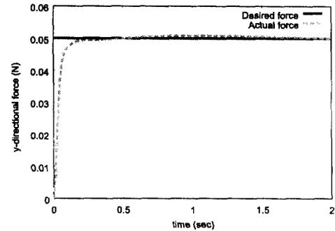
Figure 6: Force trajectory to the  $y$ -direction in case I.
