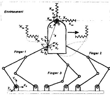
Figure 7: Compliance control by three-fingers.
