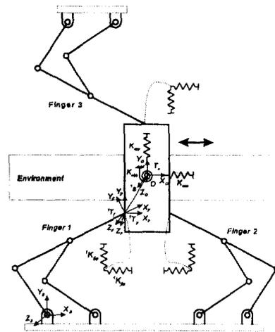
Figure 9: Compliance control by three-fingers.
