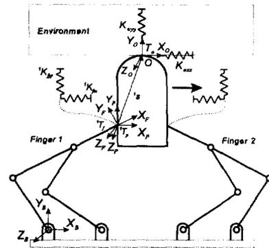
Figure 2: Compliance control by two-fingers.
