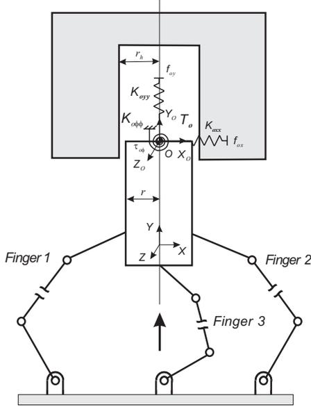
Figure 1: Peg-in-hole task using a three-fingered robot hand.
