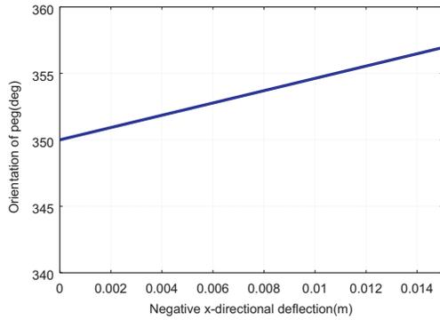
Figure 6: Orientation of the peg for left-side contact.
