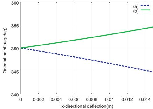
Figure 7: Orientation of the peg for right-side contact: (a) is the case that the compliance center lies in the peg tip and (b) is the case that the location of compliance center is modified.
