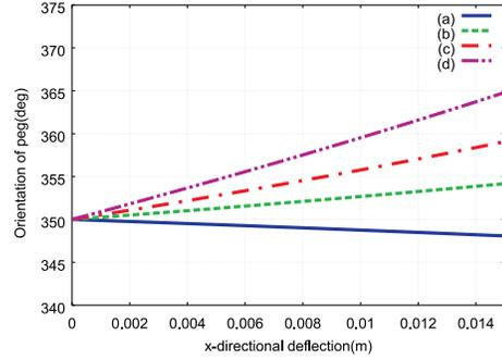
Figure 12: Orientation of the peg for right-side contact in the peg-out-hole task: (a)  $\mathcal{O}_1$  (b)  $\mathcal{O}_2$  (c)  $\mathcal{O}_3$  (d)  $\mathcal{O}_4$ .
