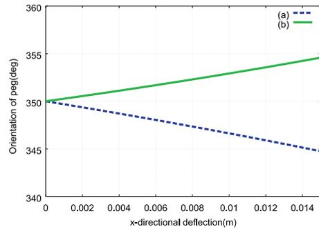
Figure 9: Orientation of the peg for right-side contact: (a) is the case that the compliance center lies in the peg tip and (b) is the case that the location of compliance center is modified.
