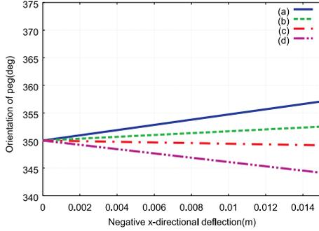
Figure 11: Orientation of the peg for left-side contact in the peg-out-hole task: (a)  $\mathcal{O}_1$  (b)  $\mathcal{O}_2$  (c)  $\mathcal{O}_3$  (d)  $\mathcal{O}_4$ .
