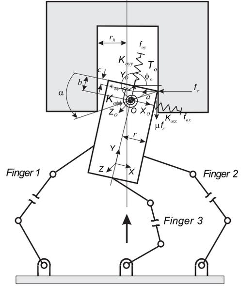
Figure 5: Modified right-side contact.
