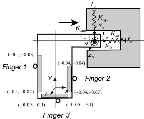
Figure 9: Peg-in-hole task with L-type object.
