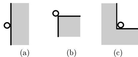
Figure 3: Types of grasp points: (a) edge (b) convex vertex (c) concave vertex.
