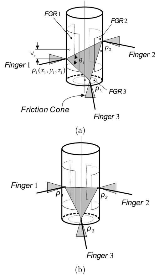
Figure 4: Grasp triangle as grasp location: (a) any point in  $FGR$  (b) center point in  $FGR$
