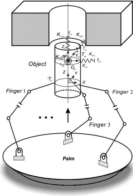
Figure 5: Peg-in-hole task by using multi-fingered hand.
