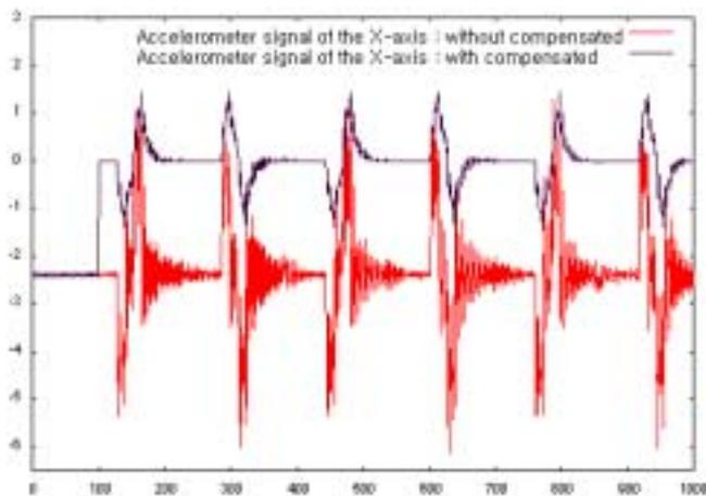
Figure 7 : Accelerometer output signal of X-axis(m/sec<sup>2</sup>)
