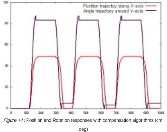
Figure 14 : Position and Rotation responses with compensation algorithms (cm, deg)
