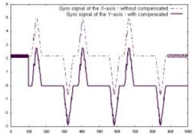
Figure 10 : Gyro output signal of Y-axis(deg/sec)
