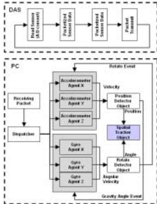
Figure 2: Spatial tracking system software structure
