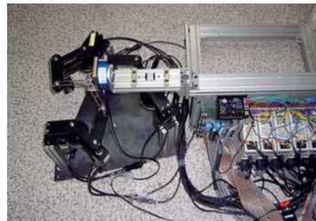
Figure 9. Prototype of 3 DOF parallel haptic device
