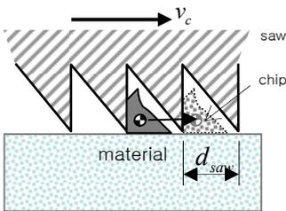
(a) Geometry of saw and chip
