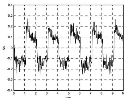
Figure 11. External Impulse Profile of Single Arm Sawing Task with Hard Material
