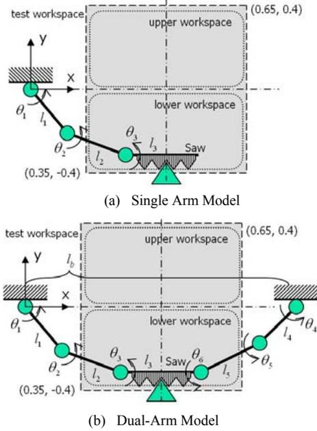
Figure 4. Models of Human Sawing Task
