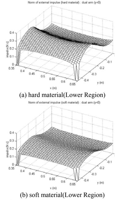
Figure 6. Distribution of External Impulse by using Dual-Arm
