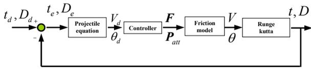
Fig. 13 Block diagram for controlling the arrival time and arrival distance of a ball
