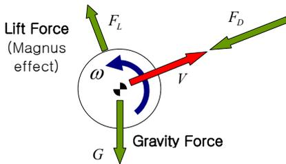
Fig. 3 Aerodynamic forces applied to a flying ball
