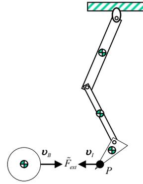
Fig. 2 Kicking model of a human leg
