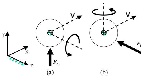
Fig. 5 Direction of the lift force according to the rotational direction
