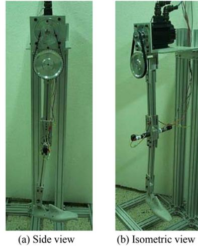
Fig. 16 Experimental Setup for Kicking a Soccer Ball
