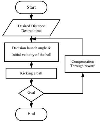
Fig. 14 Flowchart for the reinforced learning control
