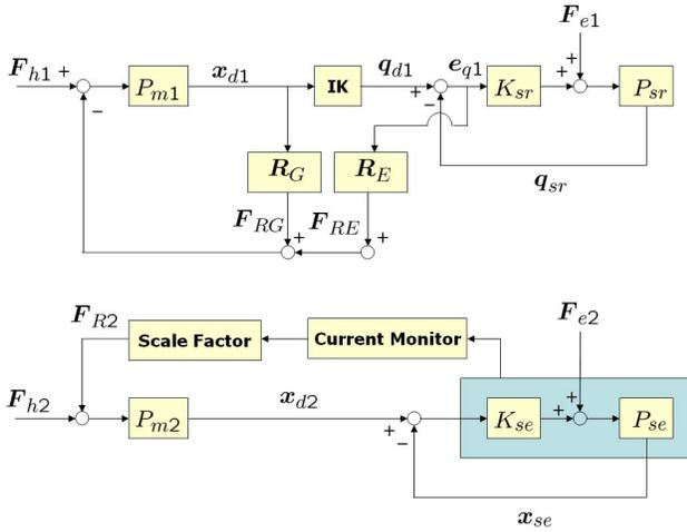
Fig. 12. Whole system diagram for BiTESS-II
