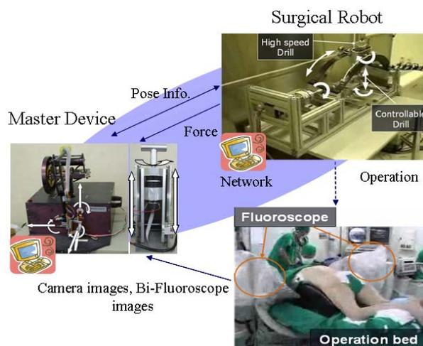
Fig. 6. Architecture of BiTESS-II
