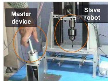
Fig. 4. 1-DOF drilling bilateral operation system.
