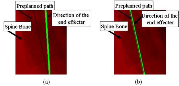
Fig. 14. Displayed images of a preplanned operation path and the direction of the end effector (the operator controls the direction of the end effector (green line) to match it to the preplanned path (black line) displayed on the spine bone image) : (a) Before operation (b) After operation.
