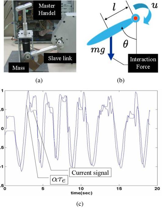
Fig. 11. Current monitoring method: (a) Experimental setup (b) Simplification of experimental setup. (c) Current monitoring Signal and calculated torque(scaled).
