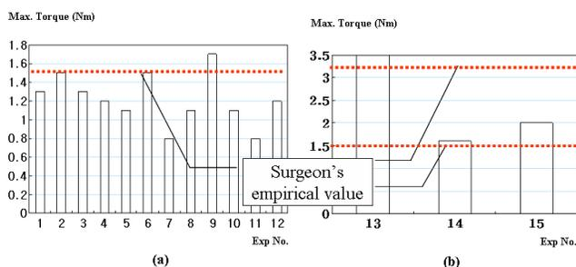
Fig. 5. Maximum torques to insert a screw: (a) Maximum torques into the sponge bone (b) Maximum torques into the sponge bone through the cortical bone.
