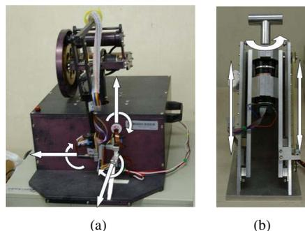
Fig. 10. Master Devices: (a) 6 D.O.F master device (b) 2 D.O.F master device.
