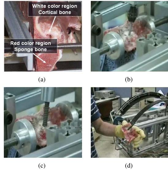
Fig. 13. Experimental results: (a) Composition of pig's spine bone (b) High speed drilling process (c) Controllable drilling process (d) End of the operation.
