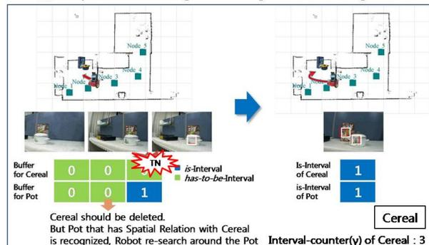
(c) False negative detection of Cereal using Action Recommendation rules
