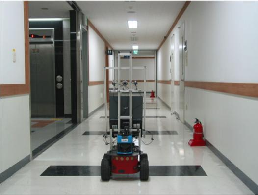
Fig. 5. Real robot platform. A Pioneer 3-AT mounted with three web cameras for image gathering.
