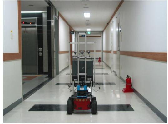
Fig. 7. Real robot platform. A Pioneer 3-AT mounted with three web cameras for image gathering.
