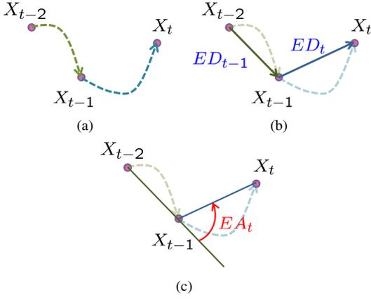
Fig. 4. Robot Motion Model : (a) Real robot motion, (b) Effective Distance ( $ED$ ), and (c) Effective Angle ( $EA$ ).
