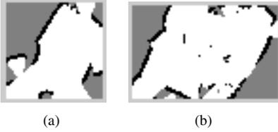
Fig. 5. Template gridmaps from node C : (a) Insufficient template gridmap to perform the reliable gridmap matching, and (b) Expanded template gridmap by accumulating more sensor data.
