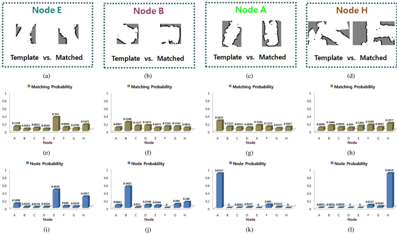
Fig. 8. Experimental results of topological localization (arranged in time sequence). (a)-(d) Template gridmaps and matching results, (e)-(h) corresponding matching probability  $P_{match}$  (5), and (i)-(l) corresponding node probabilities.
