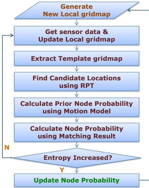
Fig. 3. Flowchart of the proposed sequential topological localization using sonar gridmap.
