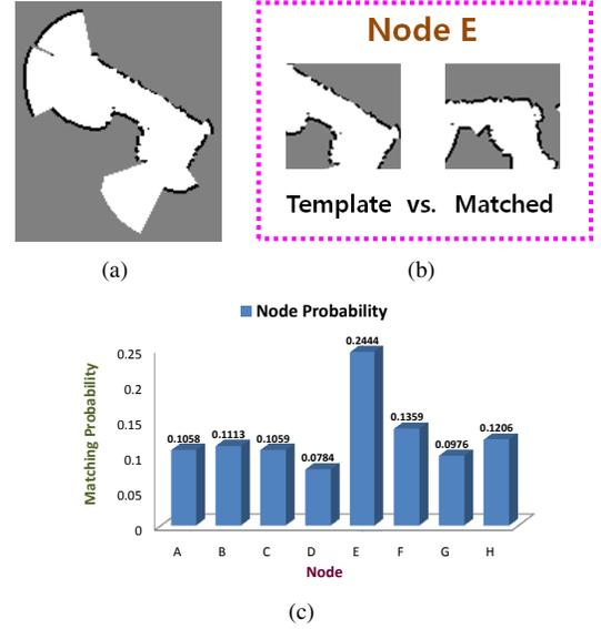
Fig. 2. Node Classification : (a) A local gridmap, (b) Template gridmap and matching result, and (c) Matching probability.
