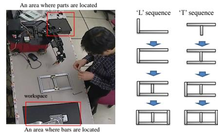
(a) Experimental setup. (b) Two typical assembling sequences.
