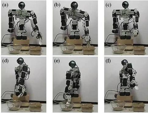
**Figure 2: Results of incrementally generating primitive skills for making coffee: (a) approaching; (b) scooping; (c) delivering; (d) pouring; (e) stirring; and (f) returning.**
