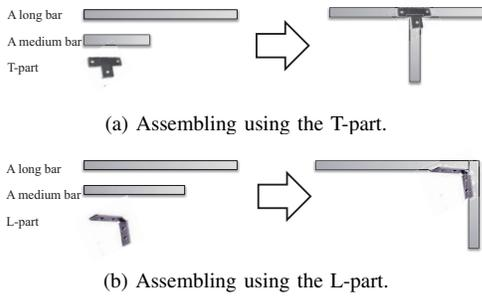
Fig. 4. Illustrations showing assemblies the T-and L-part.
