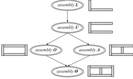
Fig. 2. An example of a temporal Bayesian network for a manual assembly task.
