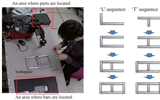
(a) Experimental setup. (b) Two typical assembling sequences.
