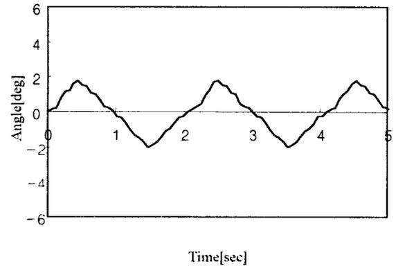
Fig. 10. Pitch motion without consideration of the internal load control.
