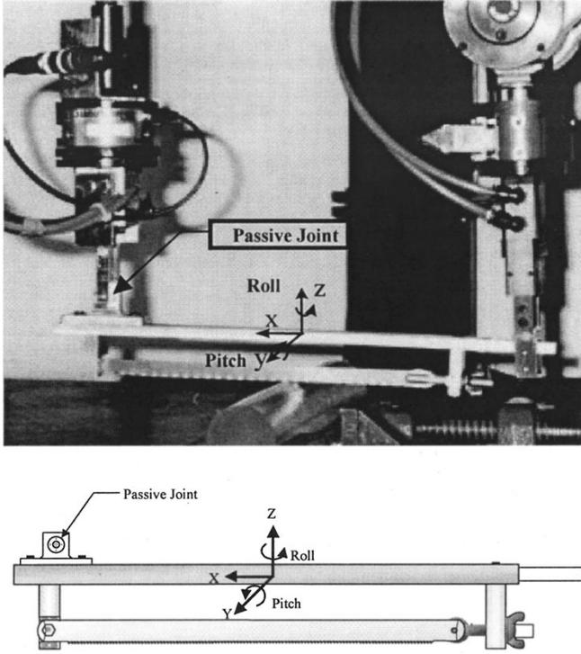
Fig. 2. A passive joint and the saw.
