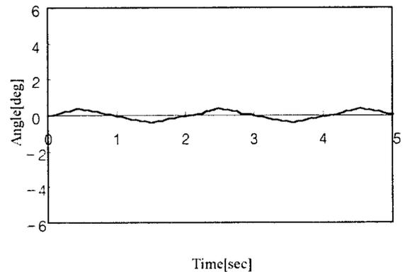
Fig. 11. Pitch motion with consideration of the internal load control.
