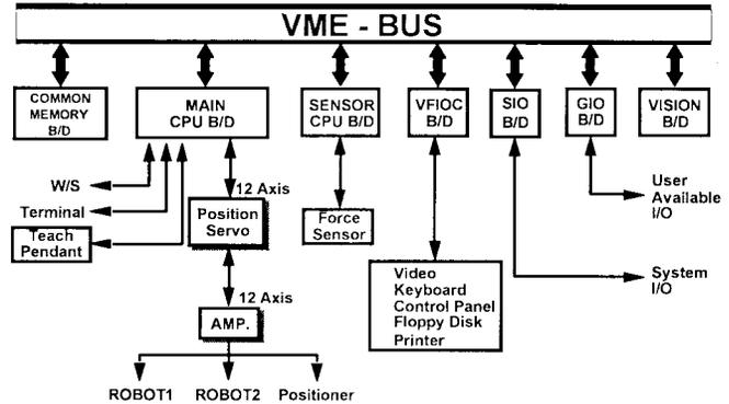
Fig. 6. Hardware architecture of the multirobot controller.
