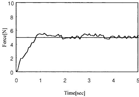
Fig. 12. Force control in the sawing task [blade type (a)].
