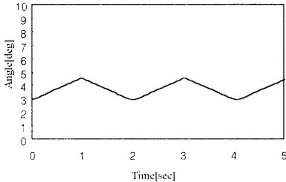
Fig. 8. Roll motion when an additional passive joint is not included.
