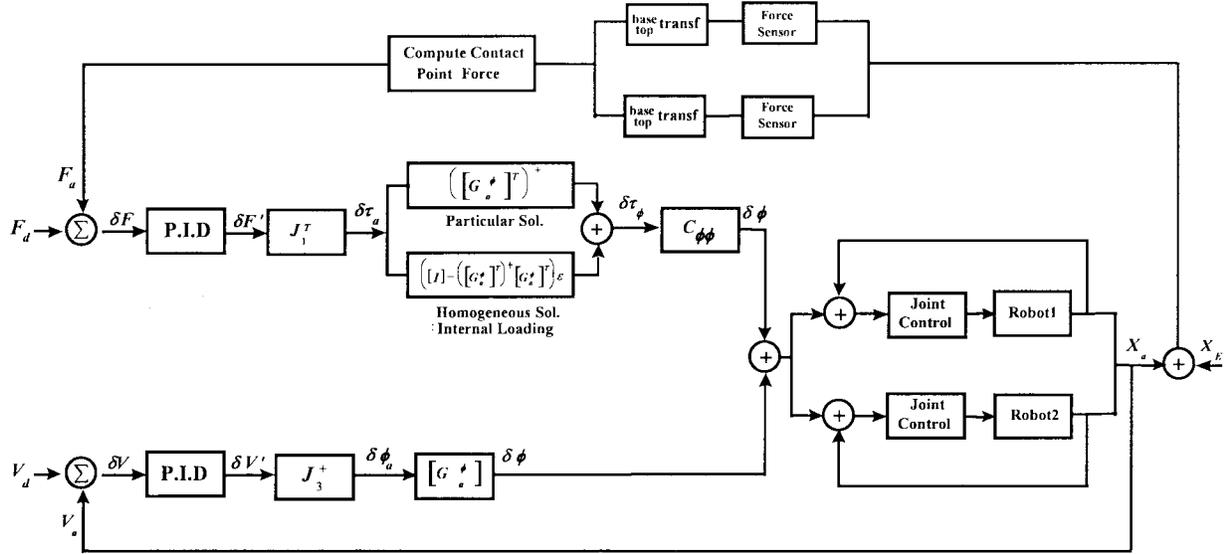
Fig. 4. Block diagram of the proposed hybrid control scheme.
