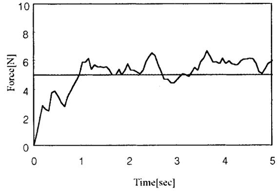
Fig. 15. Force control in the sawing task [blade type (c)].
