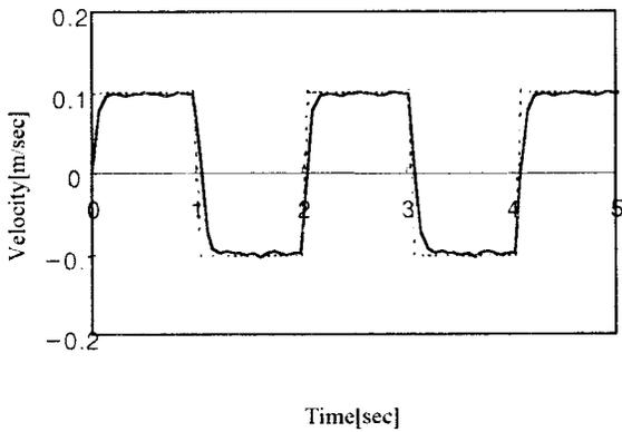
Fig. 13. Velocity control in the sawing task [blade type (a)].
