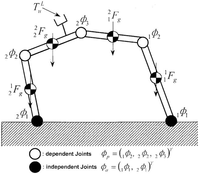
Fig. 3. Closed-loop kinematic chain.
