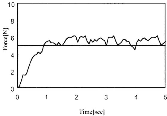
Fig. 14. Force control in the sawing task [blade type (b)].
