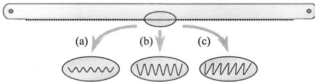
Fig. 7. Shape of saw blades. (a) Symmetric saw blade with tooth depth less than 0.1 mm. (b) Symmetric saw blade with tooth depth 0.3 mm. (c) Asymmetric saw blade with tooth depth 0.3 mm.
