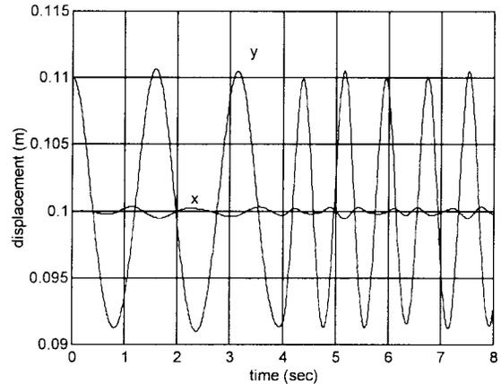
Fig. 9. End-effector motion with frequency modulation from  $\omega = 4$  rad/s to  $\omega = 8$  rad/s.
