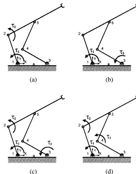
Fig. 1. Five-bar finger mechanisms.
