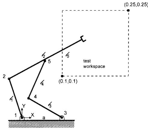
Fig. 4. Workspace of five-bar finger mechanism.
