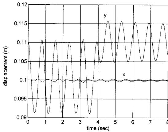
Fig. 10. End-effector motion with the equilibrium position shift from (0.1, 0.1) to (0.1, 0.11).
