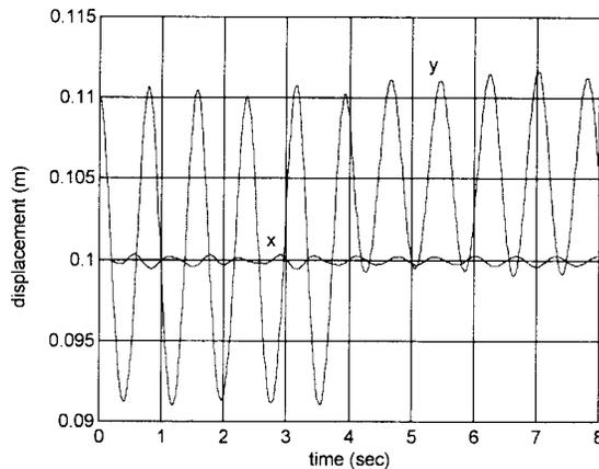
Fig. 11. End-effector motion with the equilibrium position shift from (0.1, 0.1) to (0.1, 0.105).
