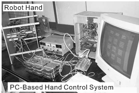
Fig. 16. Developed PC-based hand control system.
