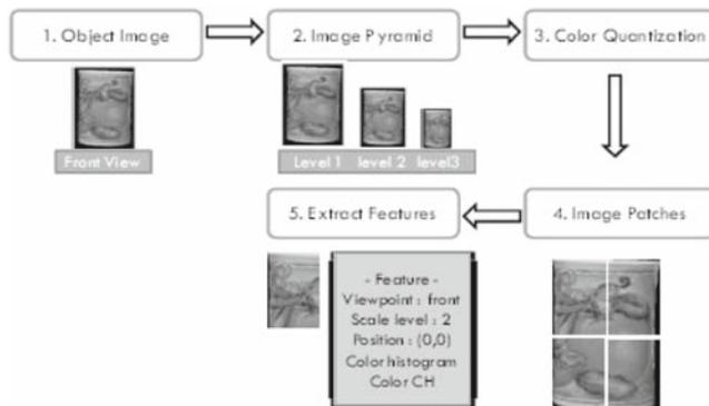
Fig. 1. Flow chart of object modeling process
