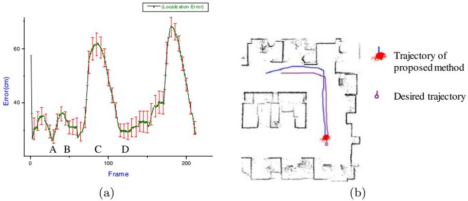
**Fig. 3.** (a) Localization errors when estimated by the spatial object contexts. (b) Localization results show the trajectory of the robot estimated by the proposed spatial object contexts.
